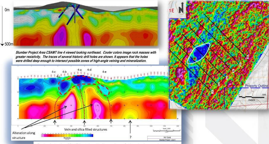
Slumber Project Area CSAMT line 4 viewed looking northeast. Cooler colors image rock masses with greater resistivity. The image shows high-angle resistive zones, surrounded by conductive rock. The blue resistive cap corresponds to silicified outcrops
